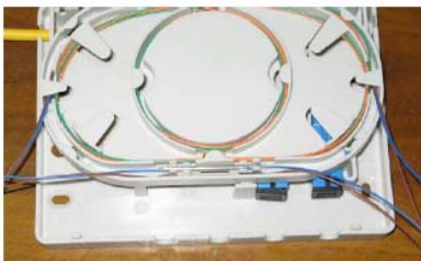
Pic14: after shrink, splice protective tube put into the slot
